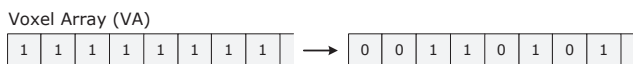
Fig. 4 Inner/outer classification of voxels. In the beginning of the second phase, the voxels in the 3D volume space, linearized into a 1D array on the GPU memory, are classified as inner (1) or outer (0) according to whether they are inside of the visual hull, i.e. whether they are inside of all the silhouette cones, generated by the extracted silhouette contours.
