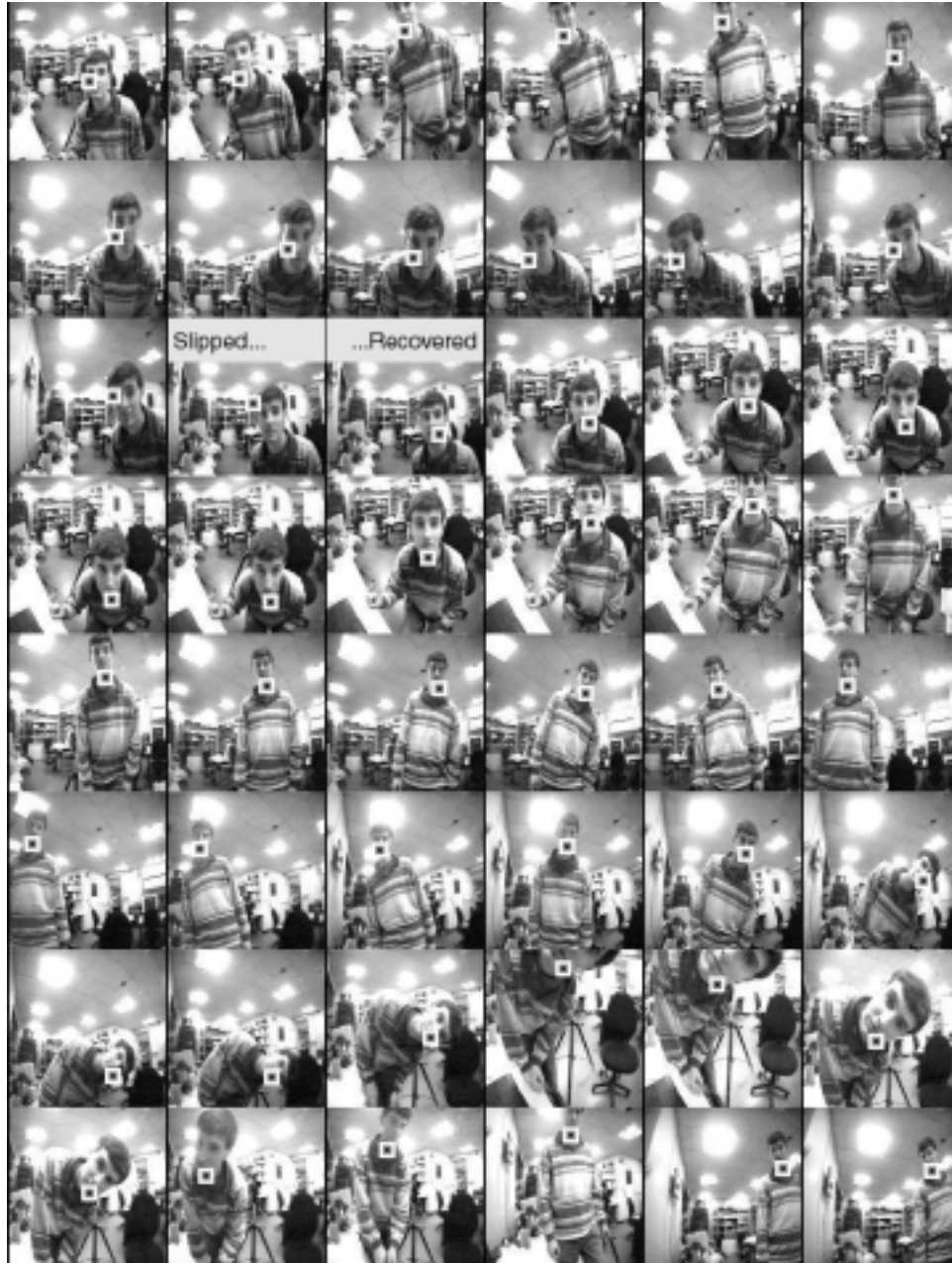
Figure 13-3: Behavior of the tracker. Frames are taken at one-second intervals. The white squares indicate the position of the target. The target is not centered in the images since they were taken from a camera fixed with respect to the head, rather than gaze direction. On the third row, the face slips away from the tracker, but it is immediately reacquired through the attention system. The images are taken from a three-minute session during which the tracker slipped five times. This is typical performance for faces, which tend not to move too rapidly.
