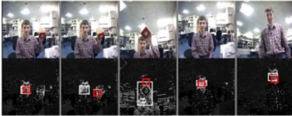
Figure 6-9: Manipulating the robot's attention. Images on the top row are from Kismet's upper wide camera. Images on the bottom summarize the contemporaneous state of the robot's attention system. Brightness in the lower image corresponds to salience; rectangles correspond to regions of interest. The thickest rectangles correspond to the robot's locus of attention. The robot's motivation here is such that stimuli associated with faces and stimuli associated with toys are equally weighted. In the first pair of images, the robot is attending to a face and engaging in mutual regard. By shaking the colored block, its salience increases enough to cause a switch in the robot's attention. The third pair shows that the head tracks the toy as it moves, giving feedback to the human as to the robot's locus of attention. The eyes are also continually tracking the target more tightly than the neck does. In the fourth pair, the robot's attention switches back to the human's face, which is tracked as it moves.
