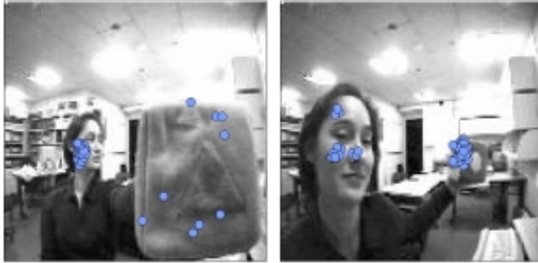
Figure 6-3: Effect of gain adjustment on looking preference. Circles correspond to fixation points, sampled at one second intervals. On the left, the gain of the skin tone filter is higher. The robot spends more time looking at the face in the scene (86% face, 14% block). This bias occurs despite the fact that the face is dwarfed by the block in the visual scene. On the right, the gain of the color saliency filter is higher. The robot now spends more time looking at the brightly colored block (28% face, 72% block).
