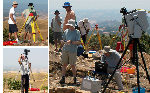
Figure 2. Research team members record exact 3D coordinates using a total station surveying instrument (upper left), capture video of an excavation using a digital camera (lower left), and scan a portion of the dig site using the Cyrax range scanner (right).
