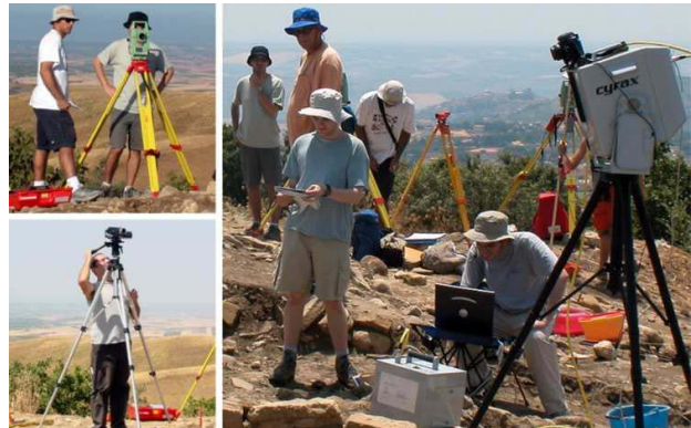
Figure 1. Members of our team record exact 3D coordinates using a total station surveying instrument (upper left), capture video of an excavation using a scanner and digital camera (lower left), and scan a portion of the excavation site using a time-of-flight laser range scanner (right).
