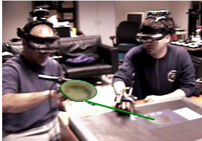
Figure 2: Two users, wearing tracked, see-through, head-worn displays and tracked 3D gloves, interact with linked 2D and 3D objects in ArchExplorer .
