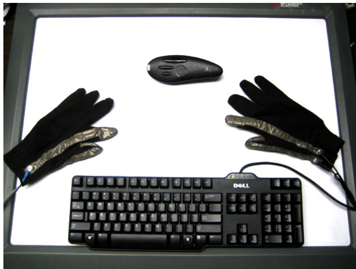
Figure 7.6: Interaction devices used in our experiment (top to bottom): A 3DOF tracked three button wand (Logitech TrackMan Live), a pair of specially constructed gloves with two active fingers on each hand, and the keyboard. The devices are laid out on the DiamondTouch surface.
