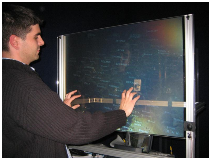
Figure 2.8: Using hand gestures to interact with map data on the TouchLight multi-touch prototype [Wilson 2004].
