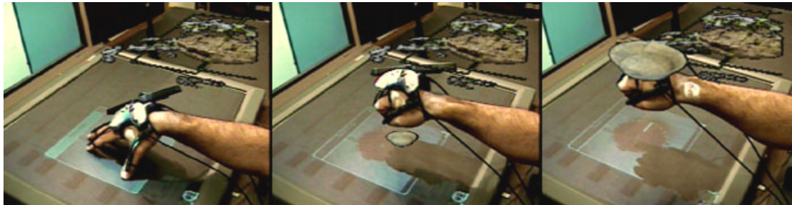
Figure 1.6: Using the Cross-Dimensional Pull gesture to transform a 2D image of a bowl found on the table into a 3D model of the same bowl above the table.
