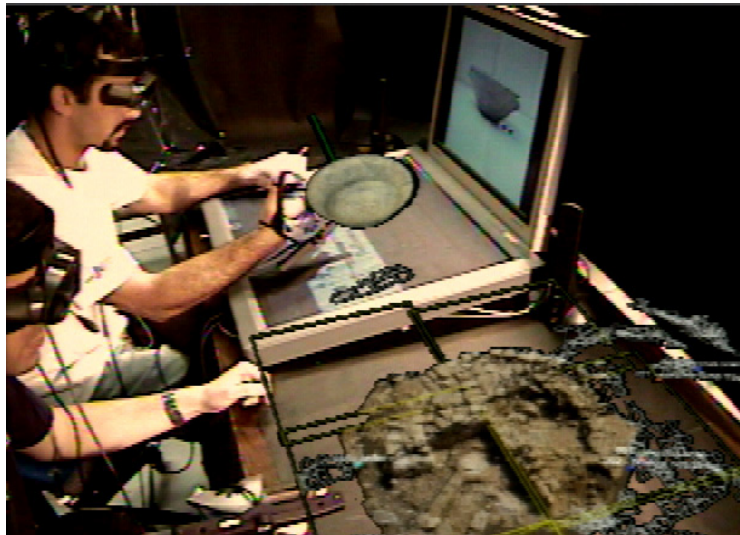
Figure 1.3: The VITA hybrid MDE [Benko 2004] (see Chapter 4) consists of four different kinds of displays: head-worn, hand-held (not shown), top-projected touch-sensitive table-top, and high-resolution vertical.
