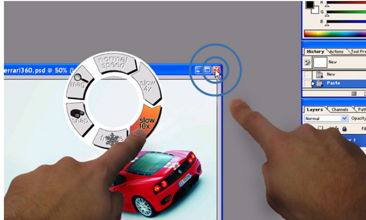
Figure 1.7: Dual Finger X-Menu technique allows the user to interactively slow down the cursor speed to improve the overall accuracy of selection.
