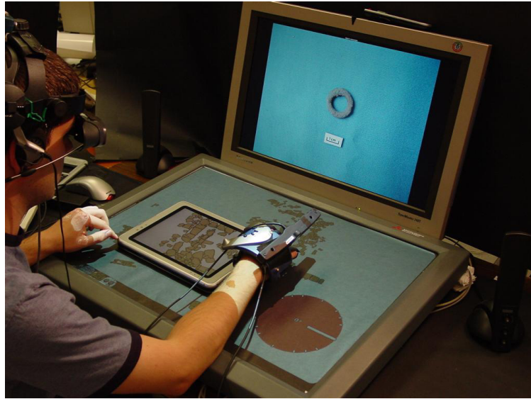
Figure 1.5: Available displays in the VITA system (left to right): tracked head-worn, projected tabletop ‡ , tracked handheld, and vertical high-resolution display.
