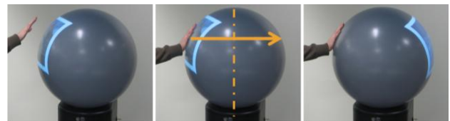
Figure 10: Send-to-Dark-Side: The user touches an object with a flat hand and waits 1 second, resulting in object being warped to the other side of the Sphere.
