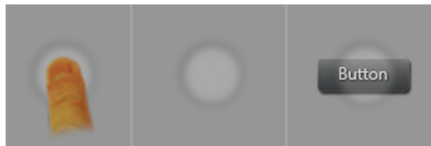
Figure 13. Rendering of Ripples contact visualization. Left: what the users see. Centre, right: what is rendered beneath the finger.
