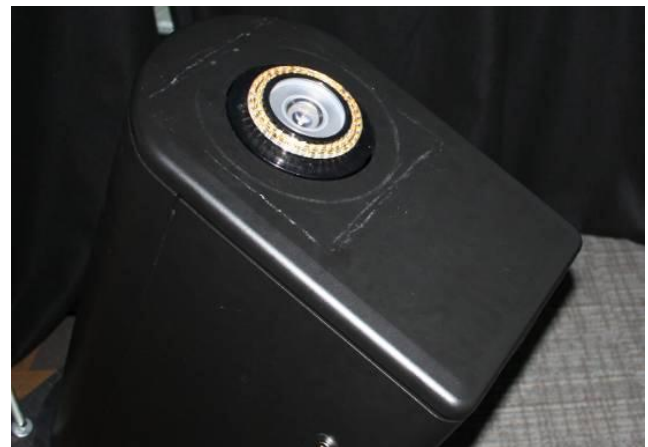
Figure 6. The projector-camera unit with a wide angle lens and infrared illumination ring. The unit is tilted 30 degrees from the vertical orientation to provide more comfortable viewing in the dome.
