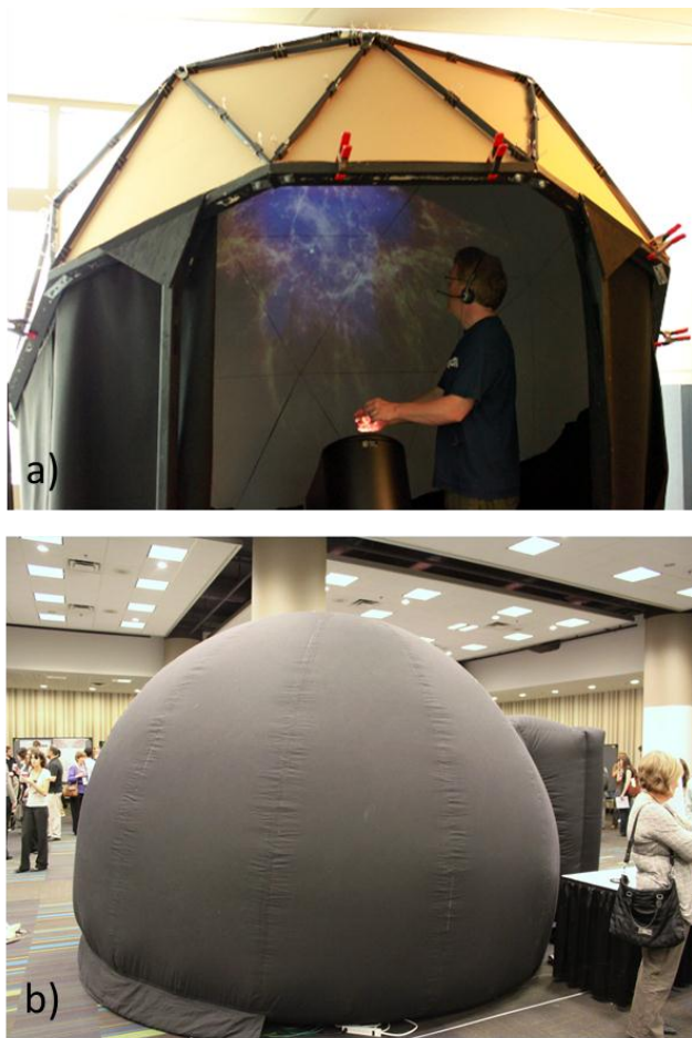
Figure 8. Two implementations of our Pinch-the-Sky Dome: a) a 9ft diameter cardboard geodesic dome and b) a 15ft diameter inflatable dome.
