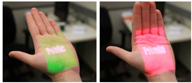
Figure 12. OmniTouch can infer if a surface is public or private from orientation features.
