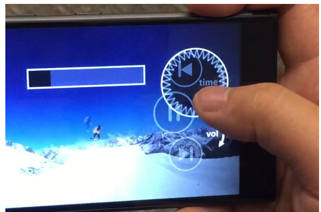
Figure 6. Dialing. The timeline and volume controls morph into dials when they fade in for one-handed interaction.
