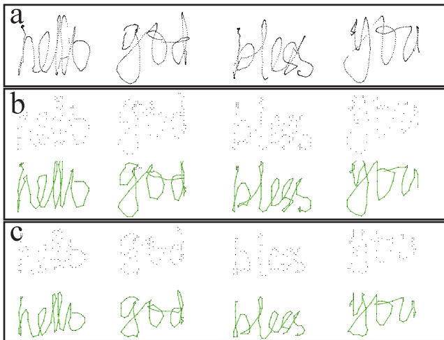
Figure 10. We demonstrate the advantages of hand writing with Hybrid HFR Depth. (a)(b)(c) are generated from the same motion sequence. The task is challenging because writing words involves many sharp turns and curves, requiring high frame rate and high accuracy. (b) illustrates using the regular Kinect depth stream (closest point), and (c) illustrates the trace of the Kinect skeleton hand tip. (a) illustrates Hybrid HFR Depth trace, which is of noticeably higher quality due to greater sampling frequency.
