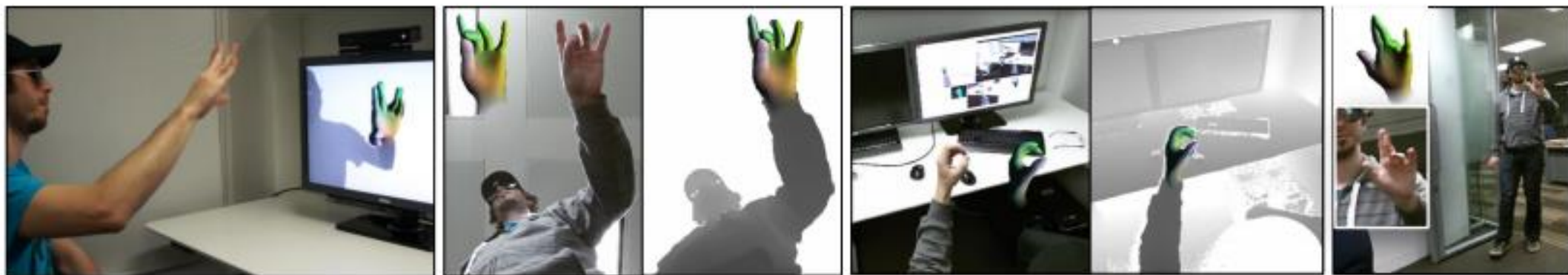
Figure 1: We present a new system for tracking the detailed motion of a user’s hand using only a commodity depth camera. Our system can accurately reconstruct the complex articulated pose of the hand, whilst being robust to tracking failure, and supporting flexible setups such as tracking at large distances and over-the-shoulder camera placement.
