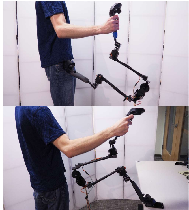
Figure 12. Grounding one controller at the waist (top) or on an external surface (bottom), to enable grounded force-feedback interactions with the other controller via the Haptic Link.
