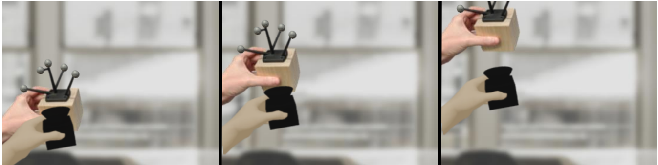
Figure 1: An illustration of the Control/Display Ratio manipulation utilized in the experiment. The user is shown lifting an optically tracked cube with the corresponding virtual representation, the movements of which are a fraction of the user's movements.
