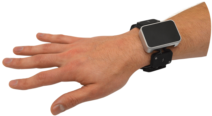
Figure 1. Tasbi is a novel multisensory haptic wristband capable of delivering squeeze and vibrotactile feedback for a variety of uses in AR/VR.
