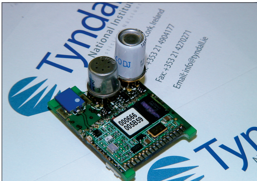
Figure 1. The 25-mm Bluetooth air-quality monitor. Onboard sensors monitor critical carbon-monoxide and volatile-organic-compound levels as well as ambient parameters such as humidity, temperature, and vibration.
