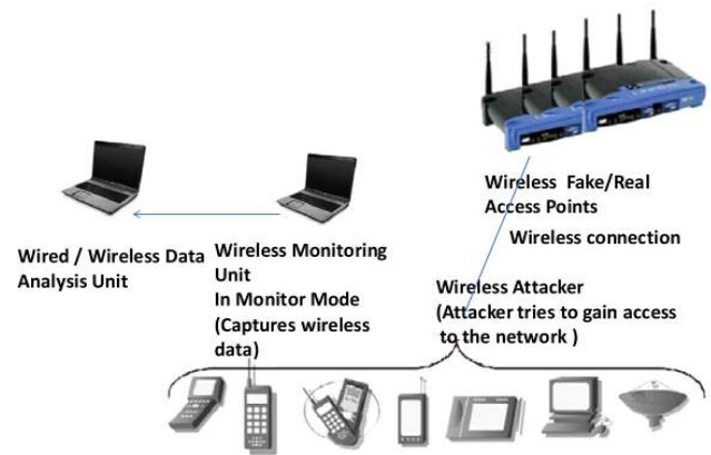
Figure 2: Honey pot based wireless network architectures for layer-2 attacks
