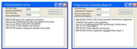
Figure 3: Background logs of the cloud platform and attacker client in the regular mobile payment process
