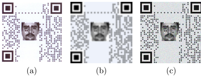
Figure 6: Results of beautified QR code of user U_1 in Table 3 after image degradation processes. (a) After Print-and-Scan attack; (b) After adding the Gaussian blurring with \sigma = 5 ; (c) After adding the Gaussian noise with parameters M = 0, V = 0.05
