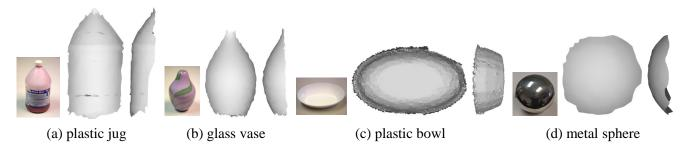
Figure 8: **Table-top objects.** We scan objects that span a variety of shapes (convex, concave) and reflectances (translucent, glossy, specular). For each object, we show a photograph under ambient light, and two views of its surface reconstruction.
