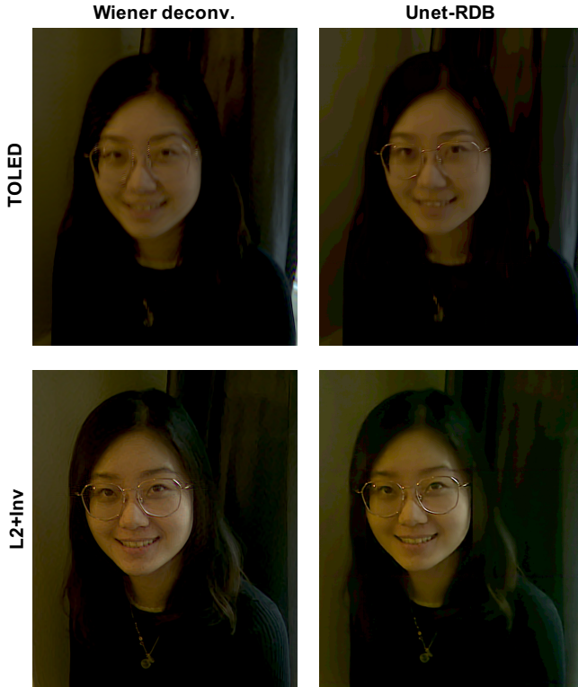
Fig. 14. Comparison of deblurring methods. We compare Wiener deconvolution and UNet-RDB on a selfie captured under conventional T-OLED and our optimized display. We use display masks of 150 DPI.
