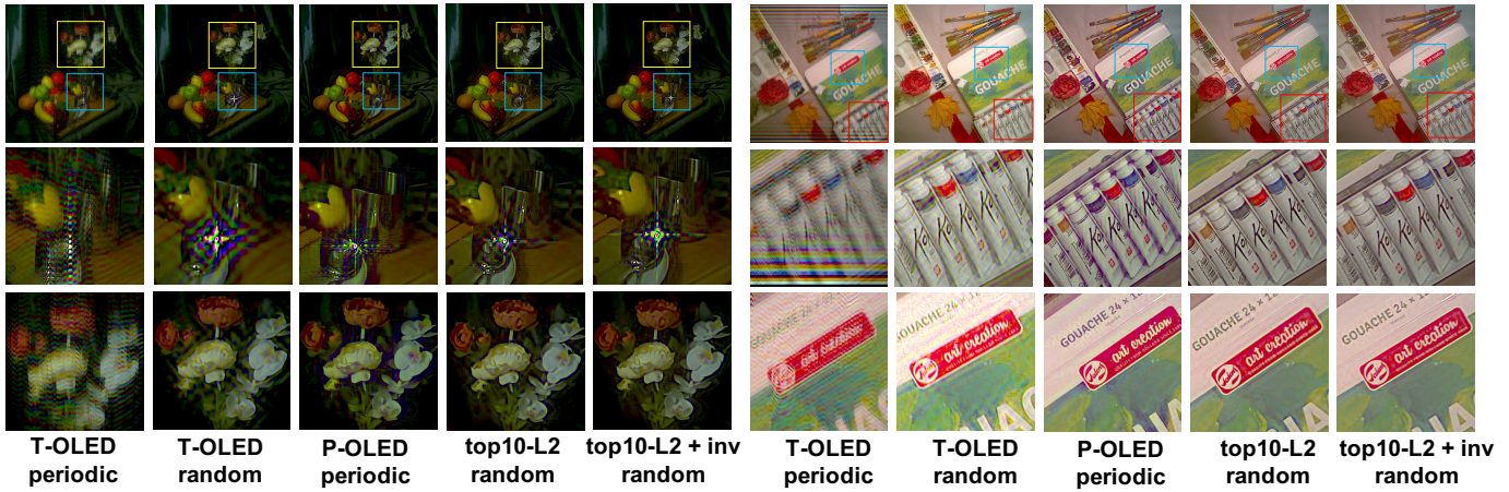
Fig. 12. Indoor scenes captured by our lab prototype under five different displays. All display masks have a pixel density of 300 DPI. We show Wiener deconvolved results. Indoor scenes are close to the camera.
