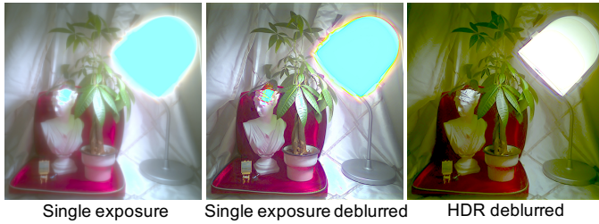
Fig. 21. Saturated regions. Saturated pixels break the linearity of the imaging model and leads to artifacts in the deblurred photograph. We alleviate these by using HDR photography to obtain a linear blur model.
