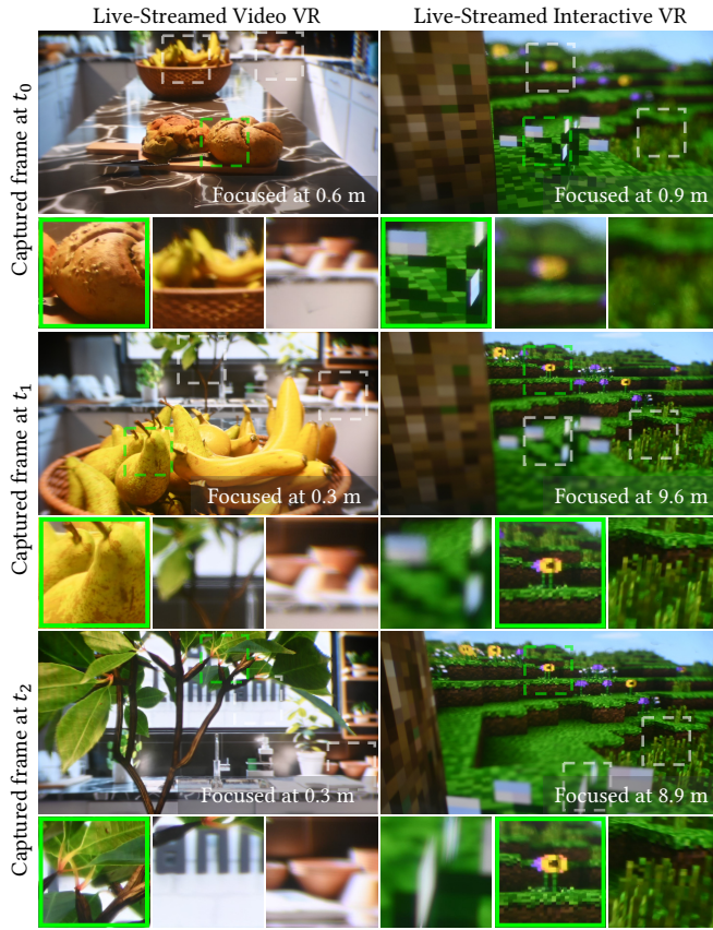
Fig. 18. A gallery of video and interactive VR results. (left) We show three frames captured with a streamed movie played on our prototype, with manual adjustment of focus. The green inset shown the region in focus in each image. We show frames from three time instances: t_0 < t_1 < t_2 . In this video, the camera is moving forward along the optical axis, and so points out of focus in earlier frame come in to focus. For example, the bananas go from out-of-focus at t_0 to in-focus at t_1 . (right) An interactive scene with a user playing the Minecraft game. As before, we manually change the focus of the camera while capturing the video game played. At t_0 , the player is standing still and our camera is focused at the near white plant. Then the camera switches focus at t_1 . The player then continued walking towards the in-focus distanced region at t_2 . (Credits: (left) "Interior Kitchen" 3D scene courtesy of "Entity Designer" at Blender Market and animation courtesy of Mohamad Zeina; (right) Craft 3D game courtesy of Michael Fogleman)
