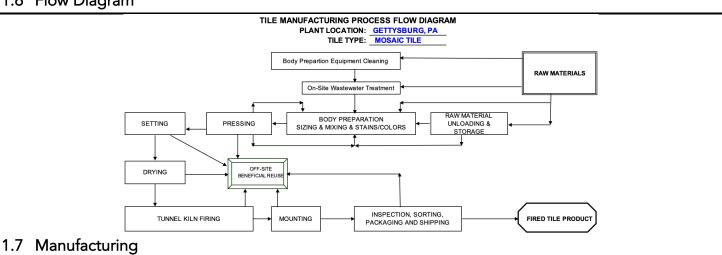
The manufacturing process begins with the mining of raw materials, which is a mixture composed mostly of clay, nepheline, kaolin, pyrophyllite and other minerals. The raw materials are mixed and grounded to a powder according to the type of tile being manufactured. Water is then added to create a body material with a moisture content suitable for extruding and/or pressing to form tiles of the
