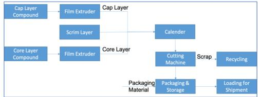
heated and pressurized and then extruded through a die to form films of a required thickness. The cap layer and core layer will join the scrim layer between a series of heated rollers. In this manner, the layers are bound together to form the final membrane. Once bound, the membrane will go through the cutter where it will be cut into specified dimensions. The finished membrane is reeled to a roll, packaged, labelled and moved into storage until it shipped to a job site for customer use.
