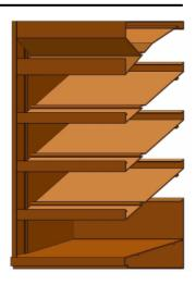
to deviate by more than 10%. Schematics of a representative type of aluminum louver (653XP) is shown here. For a full-list of available options of painted aluminum louvers manufactured by ILI please refer to: <a href="https://www.industriallouvers.com/product/?filter=fixed-extruded-drainable">https://www.industriallouvers.com/product/?filter=fixed-extruded-drainable</a>
