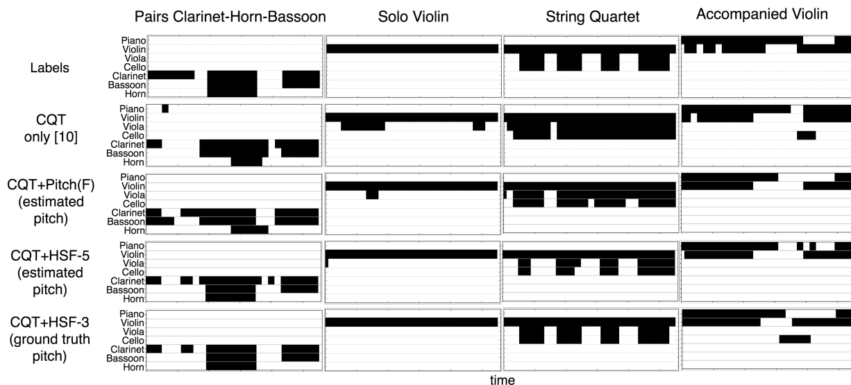
Figure 3: Prediction results of different methods for four test clips. The first row shows the ground truth frame-level instrument labels, where the horizontal axis denotes time. The other rows show the frame-level instrument recognition result for a model that only uses CQT (‘CQT only’; based on [10]) and three pitch-aware models that use either ground truth or estimated pitches. We use black shade to indicate the instrument(s) that are considered active in the labels or in the recognition result in each time frame.
