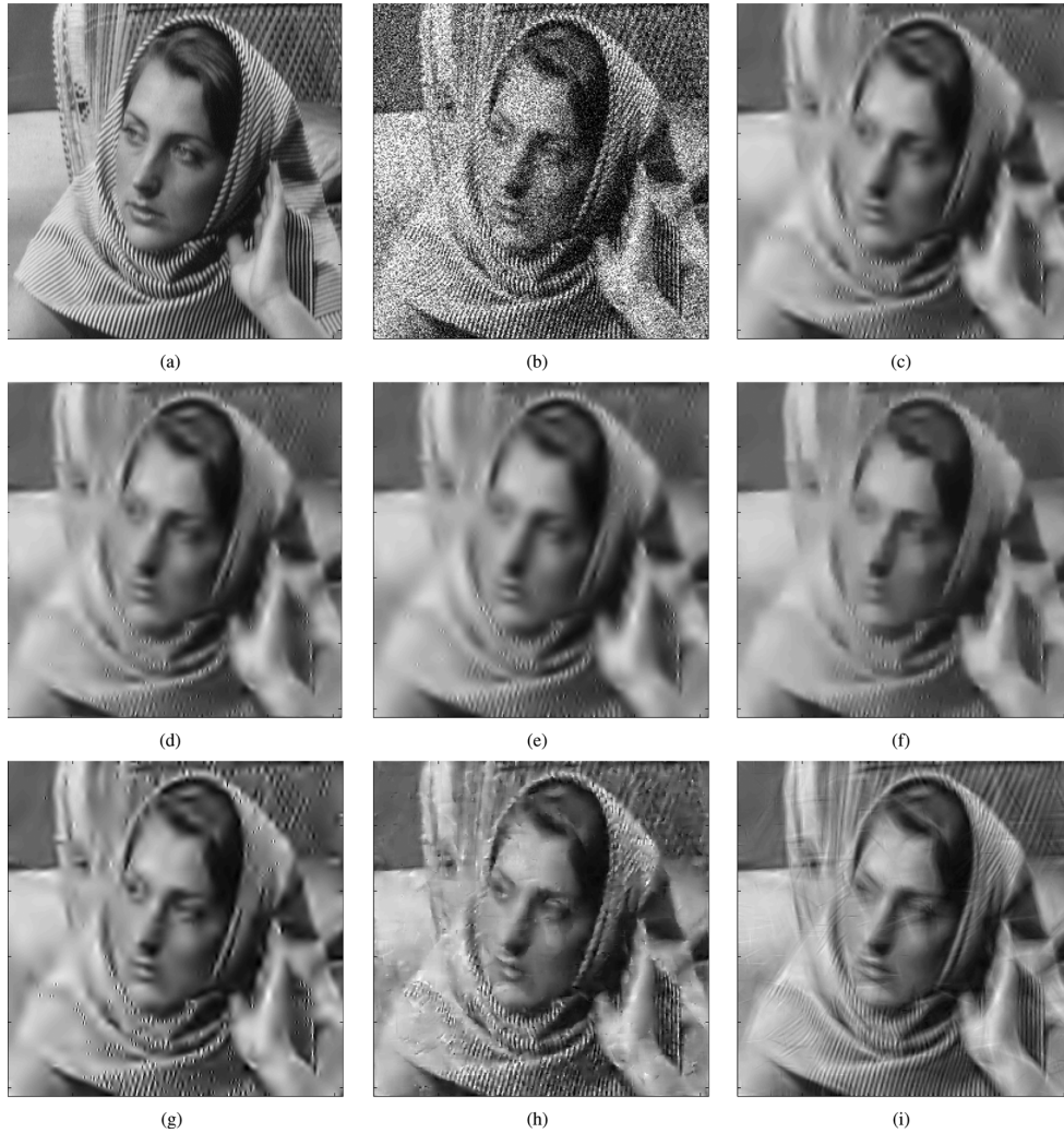
Fig. 6. Poisson denoising of the Barbara image (image size: 256 \times 256 ). (a) Intensity image (intensity \in [0.93, 15.73] ); (b) Poisson noisy image; (c) Anscombe-denoised image (UWT, 7/9 filter bank, J = 4 , FDR = 0.1, NMISE = 0.26); (d) Haar-Fisz-denoised image (UWT, 7/9 filter bank, J = 4 , FDR = 0.1, 25 cyclic shifts (five for each of the axes), NMISE = 0.28); (e) CVS-denoised image (UWT, 7/9 filter bank, J = 4 , FDR = 0.1, NMISE = 0.28); (f) denoised image by Haar+FDR (Haar UWT, J = 4 , FDR = 0.1, NMISE = 0.29); (g) denoised image by MS-VST + UWT (UWT, 7/9 filter bank, J = 4 , N_{\max} = 5 iterations, FDR = 0.1, NMISE = 0.26); (h) platelet-denoised image ( \gamma = 1/3 , 25 random cyclic shifts, NMISE = 0.18); (i) denoised image by MS-VST + curvelets ( J = 4 , N_{\max} = 5 iterations, FDR = 0.1, NMISE = 0.17).
