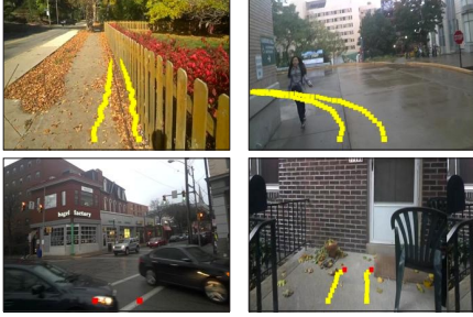
Figure 4. Example motion trajectories obtained from accelerometer and orientation sensor readings. Red dots indicate moments when the camera wearer is stationary.
