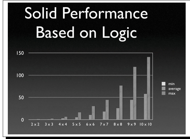
Figure 5: Performance of a RASCALS-Powered Robot in the Wumpus World. This graph shows the time (in secs) it takes the logic-powered robot to succeed in the wumpus world, as a function of the size of the world (i.e., the size of the grid). The speed is really quite remarkable. Engineering was carried out by Matt Daigle.
