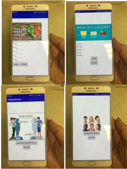
Fig. 6. Dietary System: updating dietary history (left-top), checking food information(right-top), checking eating disorder status(left-bottom), getting emotion status identification (right-bottom)
