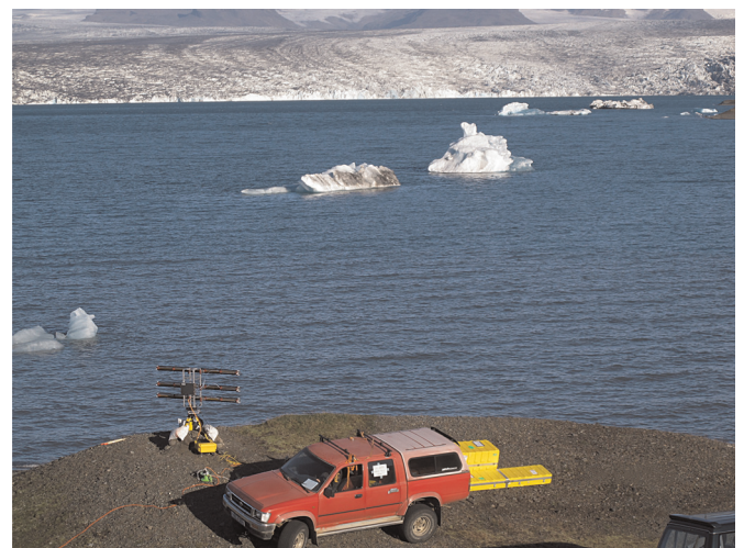
Fig. 2. A typical TRI field set-up. Since the primary purpose of the TRI is to monitor ice surface velocities, the TRI must be set up with a clear view of both the proglacial lake and of the glacier to measure ice surface velocities and to track the icebergs.
