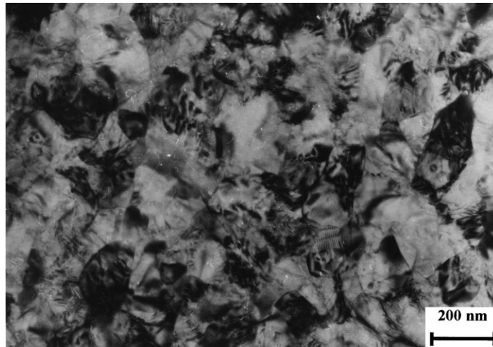
Fig. 37. TEM micrograph of titanium subjected to severe torsion straining.
