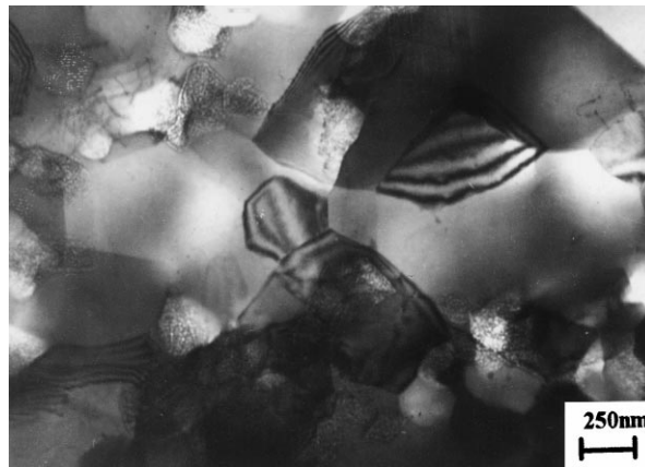
Fig. 47. Microstructure of the Al 1420 alloy after ECA pressing.
