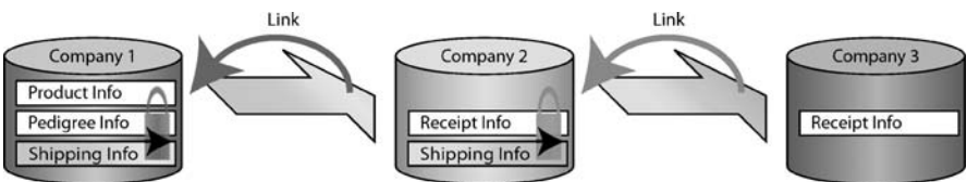
Fig. 4. A simple fragmented data approach to linking of pedigree data. Each company sends the next custodian a link to the pedigree data they hold for the product but retain the data themselves rather than embedding into a pedigree document.
