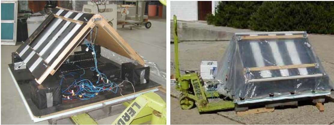
Figure 3. The Solar Tent. Left: frame with black cardboard inner roof; right: with double layer clear plastic outer roof in action.
