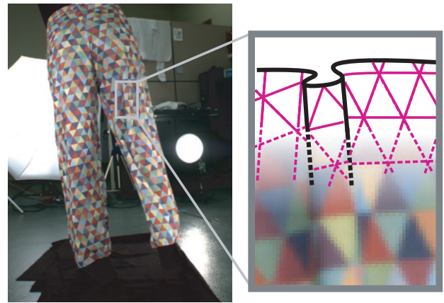
Figure 5: Neighborhood detection methods require that all markers in a fixed geometric pattern in the image neighborhood be neighbors on the cloth. Occluding contours break up neighborhood regions and limit the effectiveness of neighborhood methods in folded regions. We eliminate neighborhood requirements in the final stage of our correspondence algorithm.
