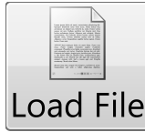
FIGURE 1.5: WPF controls are built out of composition and containment. The button shown here contains both text and an image.
