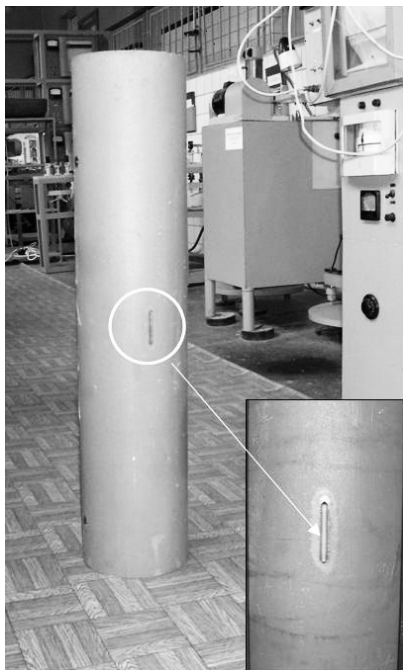
Figure 3: Notch on the pipe Slika 3: Zareza na cevi
