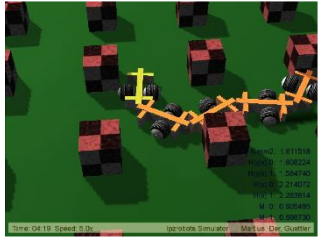
Figure 1: In the arena the chain of passively coupled two-wheel robots is simulated in the lpzrobots simulation tool. Each robot is "blind" and feels the environment only by the reactions of its wheel counters on collisions with the obstacles.
