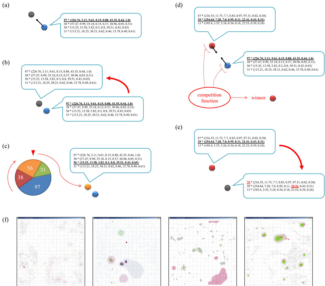
Figure 1: How particle interactions work in the revised Swarm Chemistry. (a) There are two categories of particles, active (blue) and passive (gray). An active particle holds a recipe of the swarm in it. (b) A recipe is transmitted from an active particle to a passive particle when they collide, making the latter active. (c) The activated particle differentiates randomly into a type specified by one of the kinetic parameter sets in the recipe given to it. (d) A recipe is transmitted between active particles of different types when they collide ( inheritance ). The direction of recipe transmission is determined by a competition function that picks one of the two colliding particles as a source (and the other as a target) of transmission based on their properties ( selection ). (e) The recipe can mutate when transmitted with small probability ( variation ). (f) Examples of ecologies of self-organizing patterns spontaneously formed in the Swarm Chemistry world (made of 10000 particles each).
