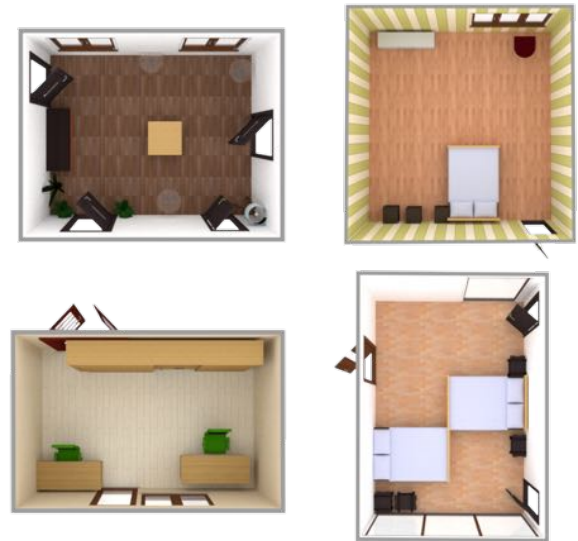
Fig. 14. Typical failure cases of our model. Clockwise from top-left: the living room contains no seats (global inconsistency), the bedroom has too many nightstands (local/global inconsistency), the wardrobe cabinet blocks the door (conflict between object location and geometry), the two beds don’t leave enough room to walk between (global inconsistency, conflict between object location and geometry).
