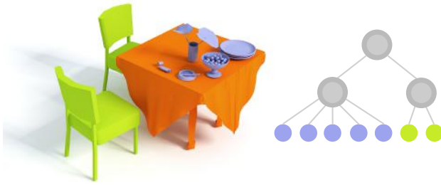
Figure 8: The ICON descriptor of the central table object shown in orange in the scene on the left. In our definition, the ICON descriptor is an object-level, geometry + interaction (GI) functionality representation. The image is courtesy of Hu et al. [HZvK*15].
