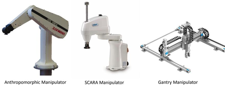
Figure 1: Serial robot examples (anthropomorphic [23], SCARA [14], gantry [22])
