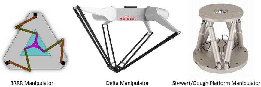
Figure 2: Parallel robot examples (3RRR [11], delta [15], stewart/gough [16])
