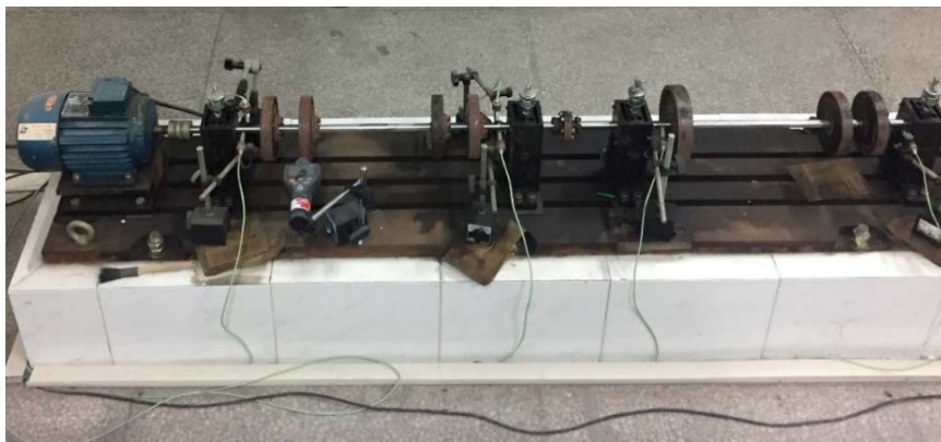
Figure 12. Structure of the gas turbine rotor testbed.
