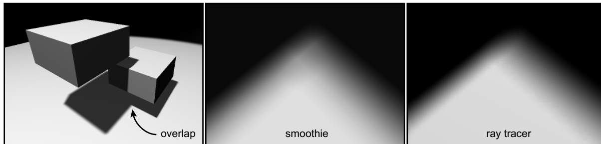
Figure 10: Comparison of overlapping penumbras. The left image shows how shadows may overlap due to multiple blockers. The next two images show a close-up of the region indicated by the arrow. The middle image is rendered using the smoothie algorithm. When multiple smoothies overlap, their alpha values are composited using minimum blending. The right image is generated using a Monte Carlo ray tracer and shows the geometrically-correct soft shadow that results from multiple blockers.
