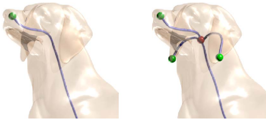
Fig. 13. Two different skeletons for the dog's head, computed, respectively, with 256 \times 256 (left) and 512 \times 512 (right) pixel silhouette images. It is our opinion that the loss of fine details in low-resolution projections reflects the behavior of human vision where the saliencies in an object are relative to the scale of observation [32].
