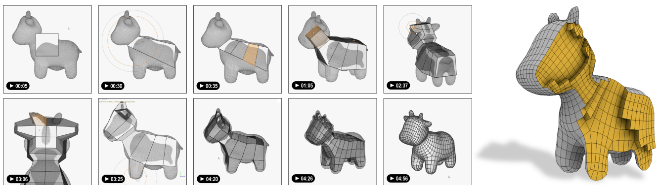
Figure 1: HexBox is an easy to use box modeling tool for hexahedral meshing. It can be used to create and project a conforming hexmesh onto a target geometry (as in this example), or to model a novel hexmesh from scratch, like in a pure modeling environment.
