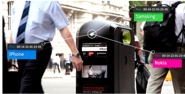
Figure 1.1: Wi-Fi bins by Renew were displaying targeted advertisements in the streets of London. Using a Wi-Fi sniffer collecting the identifiers of nearby phones, the system was able to build a profile of pedestrians and to display advertisement messages on a screen mounted on the side of the bin. These bins have been removed following a complaint by the City of London ( https://www.bbc.com/news/technology-23665490 ). Source: Renew.
