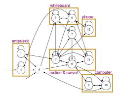
Roughly 2/3 of the transitions were trimmed. We have taken the liberty of labeling states by using forward-backward analysis to find their support in new video. The states mapped nicely to typical work activities of the office occupant. An HMM conventionally estimated from the same initial conditions is fully connected and thus too bushy to profitably illustrate or interpret.
