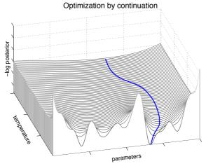
During DA, entropy at high temperatures keeps the system from prematurely committing to nearby local optima and forces it to explore the energy surface's large-scale
