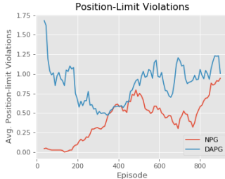
Figure 10: Safety violations observed during the training of the DClawScrewFixed task
